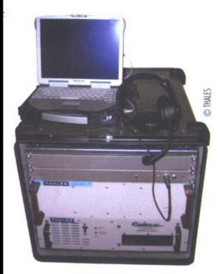
The Force Protection Jammer (FPJ) designed by Thales. It is basically an "intelligent" radio communication jammer aimed at protecting land convoys against remotely detonated mines or voice communications between forces placed in ambush.
