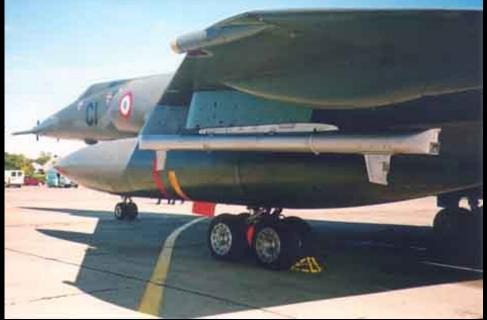
Barax NG jamming pod seen under the left wing of a FAF Mirage IVP at Cazaux Air Base last September 2002.
